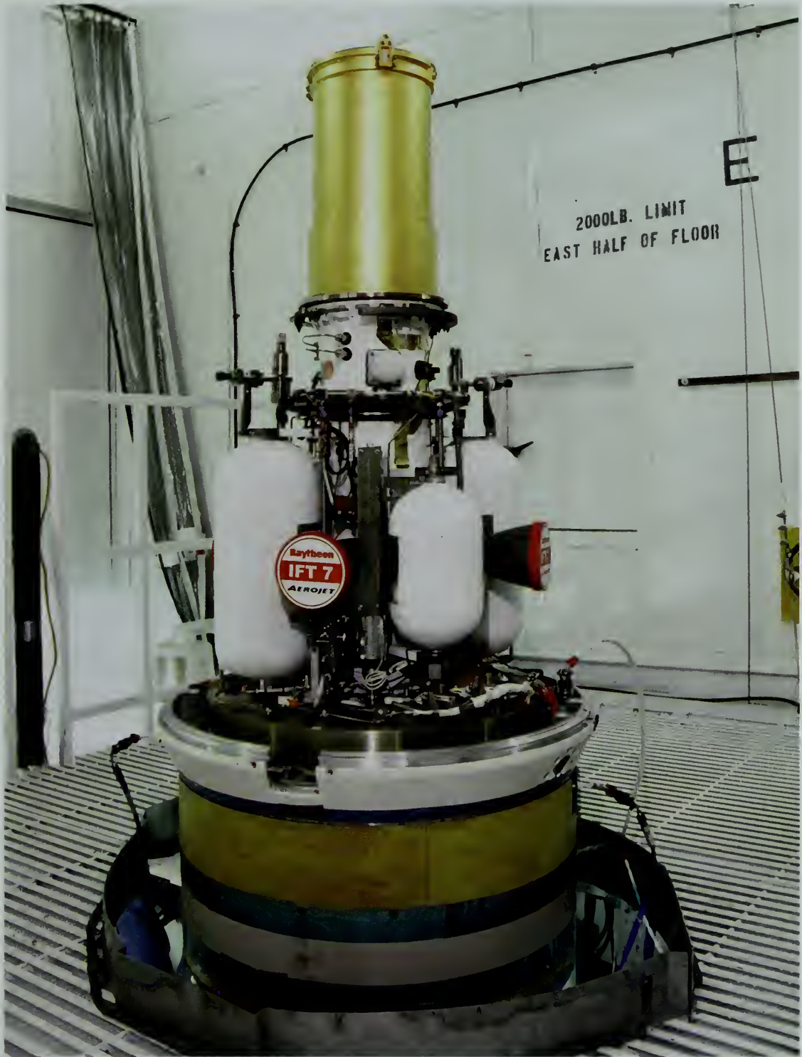
Fig. 6-18. The 121 pound Raytheon (Hughes) Exoatmospheric Kill Vehicle is navigated by an inertial navigation system updated exoatmospherically by star sightings.
